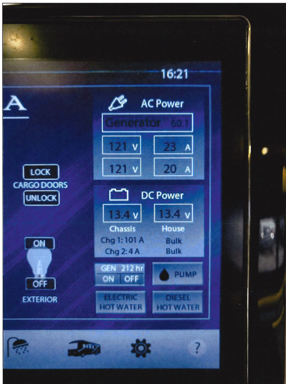
Battery Voltage Level
